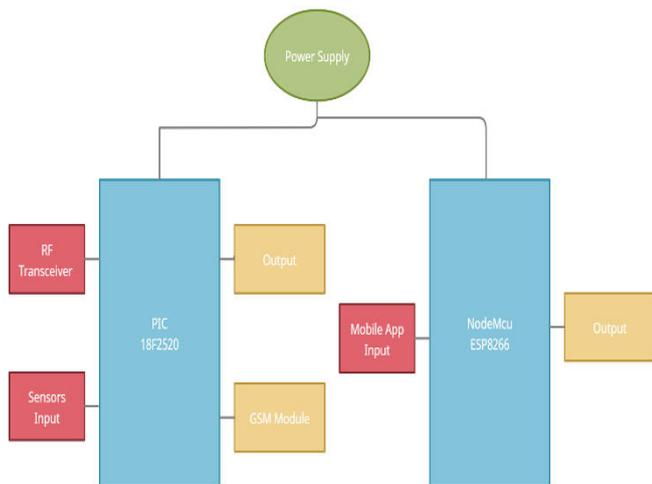
**Fig 1.** Block diagram of Multiple Sensors fault detection and monitoring system using PIC, GSM, and IoT
