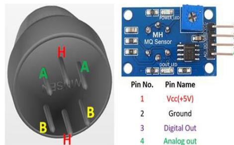
Fig 7. MQ-2 Sensor
