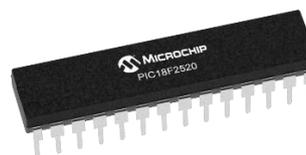
**Fig 3.** Pic 18F2520 Microcontroller
