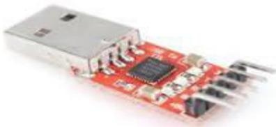
**Fig 10.** USB to TTL converter
