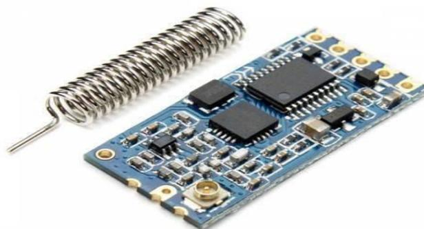
Fig 8. HC12 RF Transceiver module
