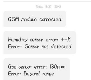
Fig 14. SMS example sent to the admin by GSM module.
